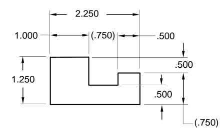
Reference dimensions are used on drawings to provide support information only.
