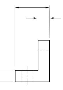
Arrowheads are used as terminators on dimension lines. The points of the arrowheads on leader lines and dimension lines must make contact with the feature object line or extension lines which represent the feature being
