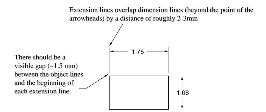
Dimensions should be placed *outside* the actual part outline. Dimensions should not be placed within the part boundaries unless greater clarity would result.
