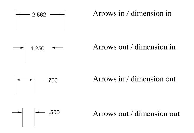
When there is not enough room between the extension lines to accommodate either the dimension value or the dimension lines they can be placed outside the extension lines as shown in the fourth example (use Flip Arrows in ProE). Reference Dimension Symbol (X.XXX)
